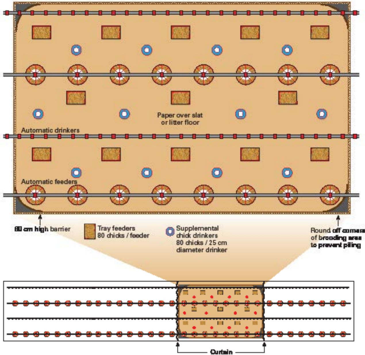
Partial house brooding provides uniform temperature to chicks
